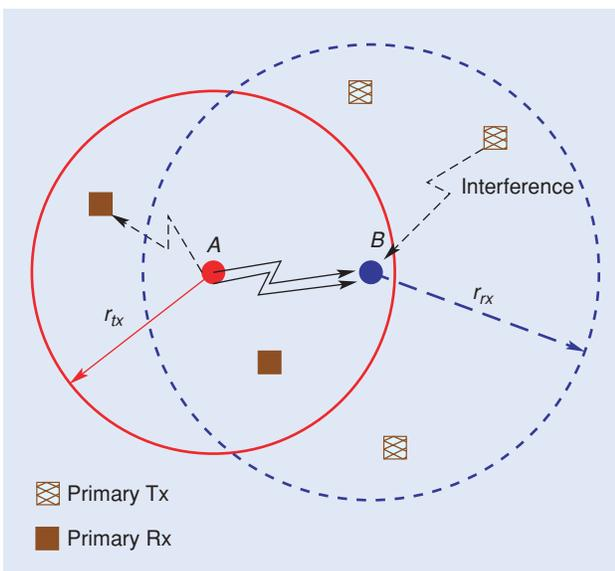
**[FIG2]** Illustration of spectrum opportunity (secondary user  $A$  wishes to transmit to secondary user  $B$ , where  $A$  should watch for nearby primary receivers and  $B$  nearby primary transmitters).
