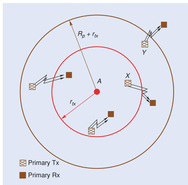
**[FIG3] Spectrum opportunity detection: A conservative approach that transforms the problem of detecting primary receivers to detecting primary transmitters.**
