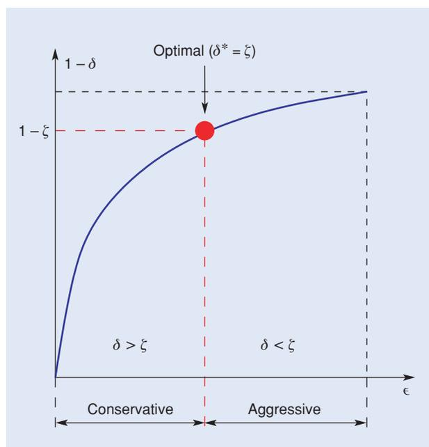
**[FIG6]** The optimal access strategy should take into account the operating characteristics of the spectrum opportunity detector ( $\epsilon$ : probability of false alarm,  $\delta$ : probability of miss detection,  $\zeta$ : maximum allowable collision probability).
